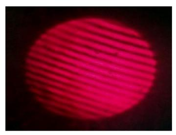
The relationship between the number of revolutions of the reducer ds, the total displacement of the flat mirror, the wavelength  $\lambda$  and intensity of the laser beam, and the enumerated maxima is as follows:
