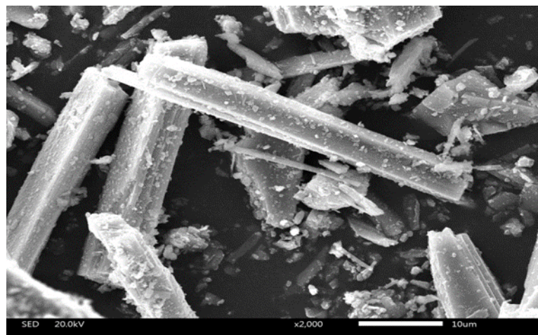
Fig. 1. Microstructure of wollastonite fiber (x2000).
