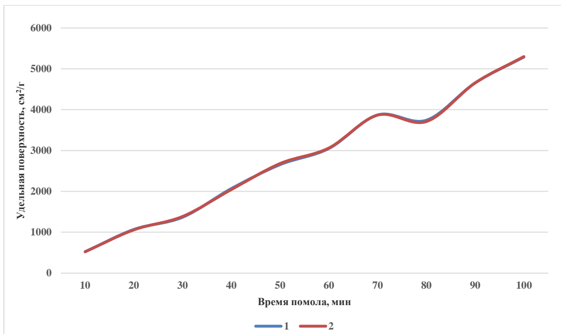
Pic. 2. Graph comparing the experimental (1) and calculated (2) values of the specific surface of the LPO obtained in the shock-attrition mode
