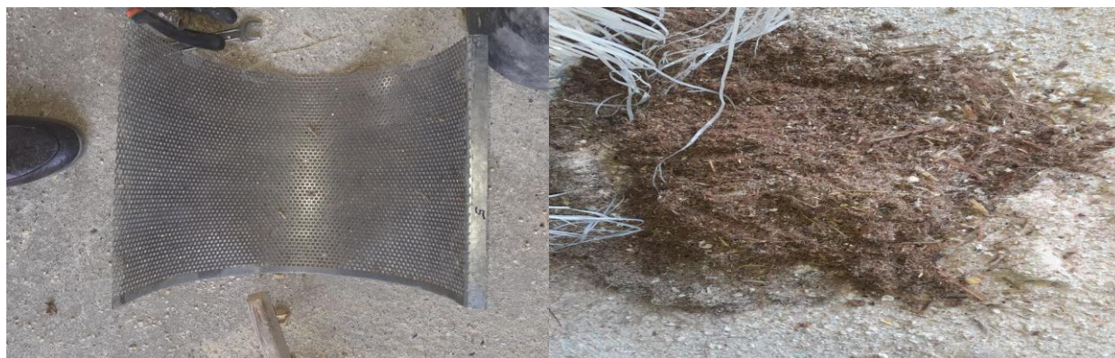
Fig. 2. Cotton stalk after grinding (milling).
