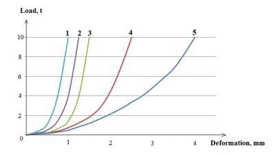
Fig.1 Graph of rubber deformation depending on the dynamic load for gaskets with a thickness of 1-7 mm; 2-14 mm; 3-21 mm; and static for gaskets with a thickness of 4-14 mm; 5-28 mm.
